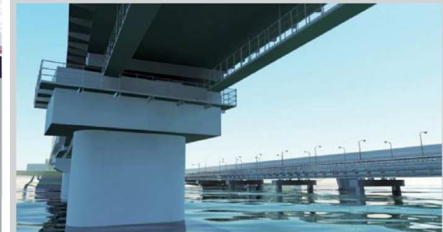
橋梁CIM (設計、施工計画) モデル CIM model of design and construction planning for bridges
